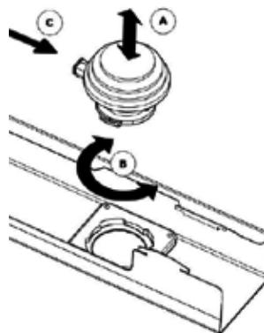
A. Fit the new LED light in the bayonet ring
