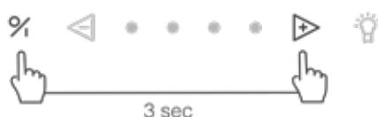
To switch the InTouch function off press the ① and ② keys at the same time for 3 seconds and the 2nd and 4th LEDs flash 3 times to confirm. (The appliance must be switched off).
