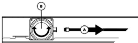
A. First disconnect the cable that runs to the LED to be replaced. Disconnect by loosening the lock by exerting slight pressure while pulling loose.
